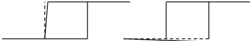
Figure 5. Potential alignment problems: (left) one of the components does not steer the beam by 90-degrees; (right) the input beam is not aligned with the breadboard. Both cases will be enough to preclude observing interference.
