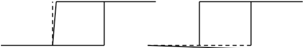
Figure 5. Potential alignment problems: (left) one of the components does not steer the beam by 90-degrees; (right) the input beam is not aligned with the breadboard. Both cases will be enough to preclude observing interference.
